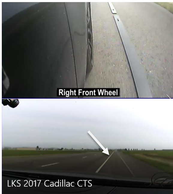
Figure 5. Point of maximum lateral deviation observed during a right-side approach test performed with the Cadillac CTS LKS and a 0.7 m/s lateral velocity
