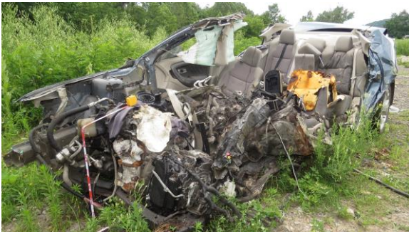
Figure 24. CISS Case No. 1-28-2017-032-01 front end crush of subject vehicle
